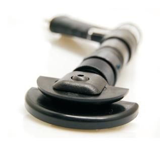
The Bend-it system is a European wide patented panel bending or crimping system driven by compressed air.
